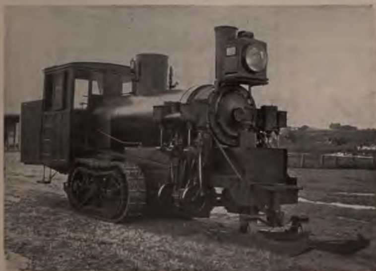
FIG. 42. — A Lombard Steam Log Hauler.
